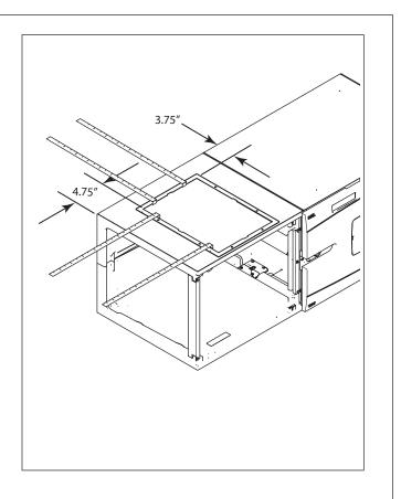
Use a felt pen to mark the 8 holes in the template.
