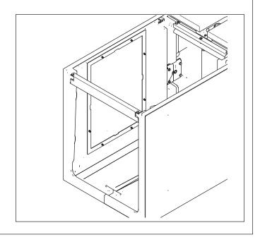
$\ensuremath{\textbf{STEP 5}}$  - Drill out the three holes located on each side of the template
