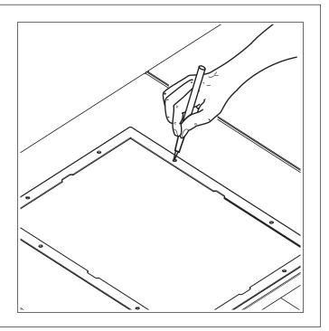
Use a 1/4 inch bit to drill each of the 8 points. The drill must be perpendicular to the air handler. The plate assembly will not fit through the holes if they are drilled in at an angle.
