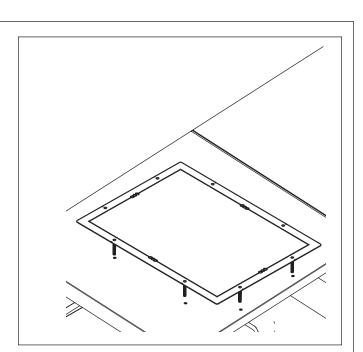
Place the template over the studs and secure with the nuts provided.
