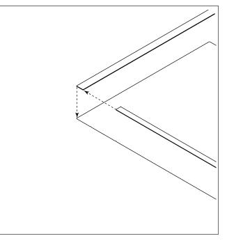
**STEP 5** - Attach the plate to the bottom of the air handler. Press firmly to make sure the double-sided tape adheres to the air handler.
